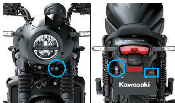
図5 GPSおよび前後カメラ Fig. 5 GPS and both front and rear cameras
