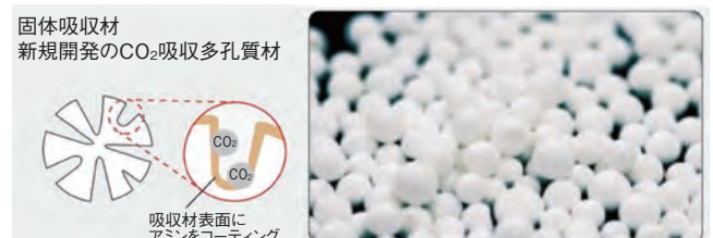
図3 固体吸収材 Fig. 3 Amine-impregnated solid sorbent
