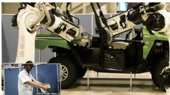
図1 一人の作業者が複数台のロボットを遠隔で操縦 Fig.1 Multiple robots remotely controlled by one worker
