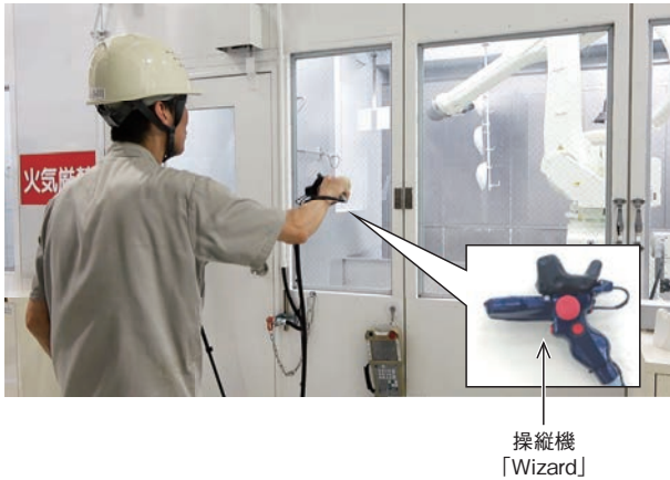
図4 塗装作業用「Successor」での塗装作業 Fig. 4 Painting operation using Successor adapted for coating
