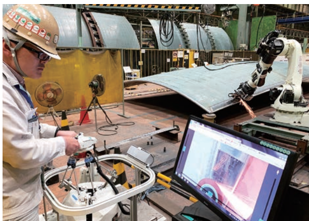
図5 「Successor-G」での研削作業 Fig. 5 Grinding operation using Successor-G
