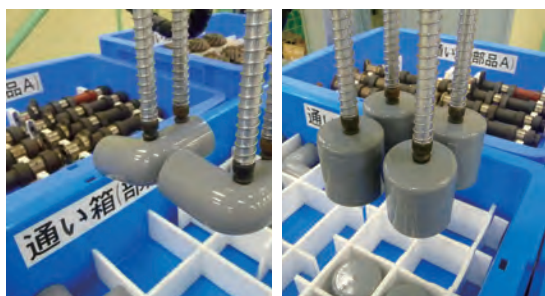
図10 吸着把持 Fig.10 Holding by suction
