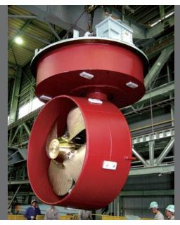
Azimuth thruster Rexpeller®
