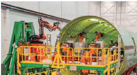
Fig. 4 Final assembly using robots (at Boeing)
