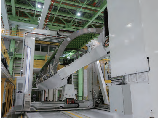
Fig. 8 Enhancement of automation using a riveting machine
