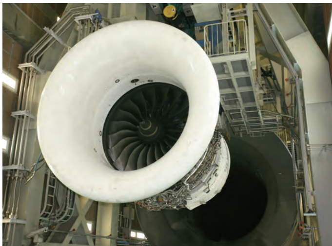
Fig. 7 Trent engine in test cell
