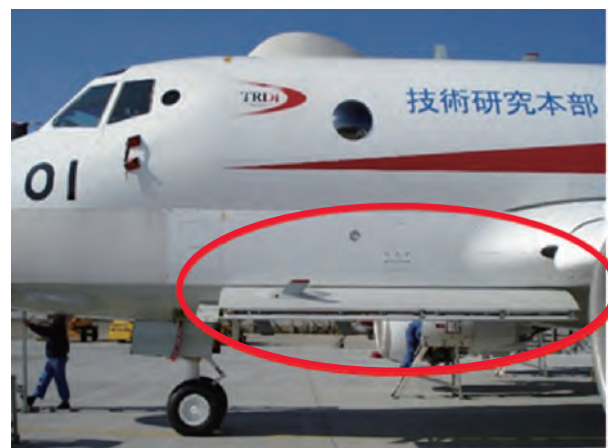
Fig. 1 Example of internal weapons bay (P-1)
