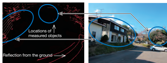
Fig. 5 Comparison between data acquired by radar and photo
