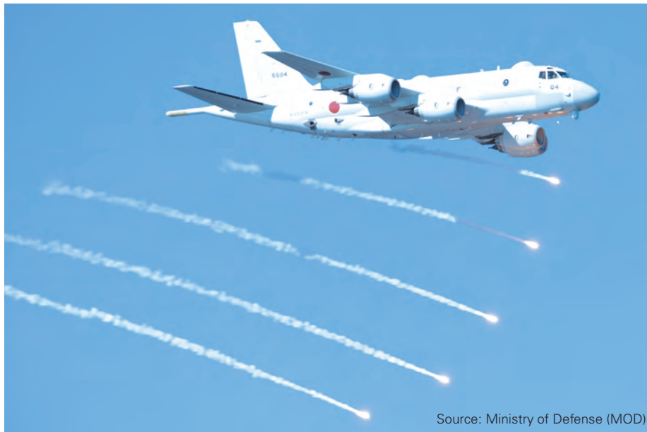
Fig. 1 Avoiding missiles by deploying flares
