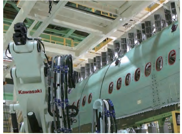
Fig. 13 Large-diameter boring robot system
