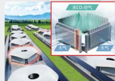
DAC (Direct Air Capture=直接空气捕集)
