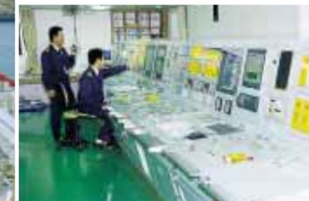
The cargo control room on board the ship is equipped with an integrated monitoring and control system (IMCS) developed by Kawasaki. It enables monitoring and control of cargo handling operations as well as monitoring engine conditions.
