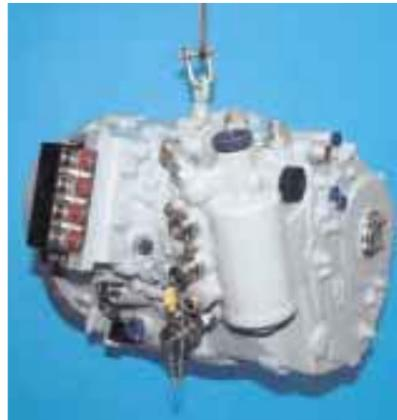
aircraft, as well as a highly-responsive electro-hydraulic servo system used to control traction drive speed, thereby ensuring superior power supply quality while allowing for uninterrupted switching of power supplies.
