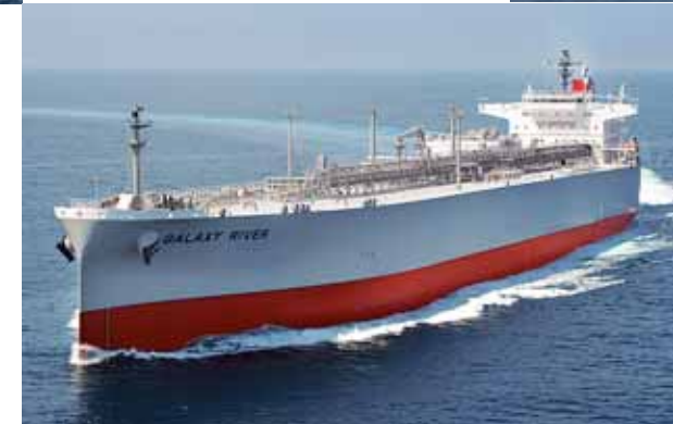
GALAXY RIVER Length/230.00m Breadth/37.20m Depth/21.00m Draft/11.20m Tank capacity/82,391m 3 DWT/54,081t Delivery/2014
