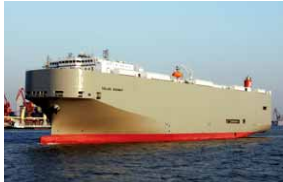
DALIAN HIGHWAY Length/199.90m Breadth/32.26m Depth/34.35m Draft/10.00m Car capacity/6,249 DWT/21,616t Delivery/2011
