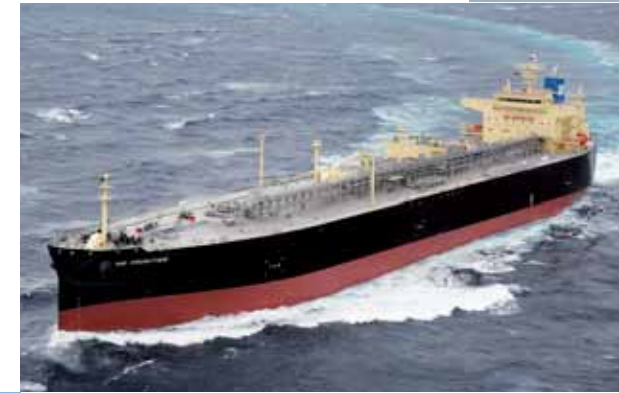
NS FRONTIER Length/229.90m Breadth/37.20m Depth/21.00m Draft/11.20m Tank capacity/82,402m 3 DWT/54,312t Delivery/2016
