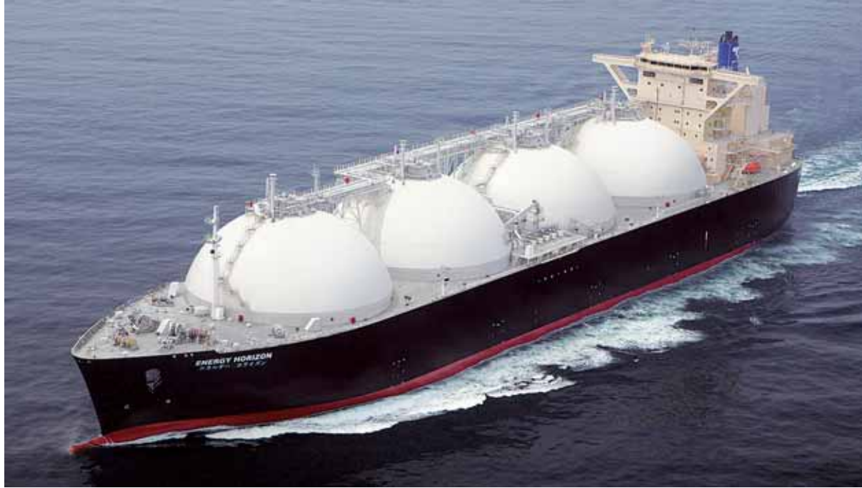
ENERGY HORIZON Length/300.00m Breadth/52.00m Depth/28.00m Draft/11.65m Tank capacity/177,440m 3 DWT/87,257t Delivery/2011
