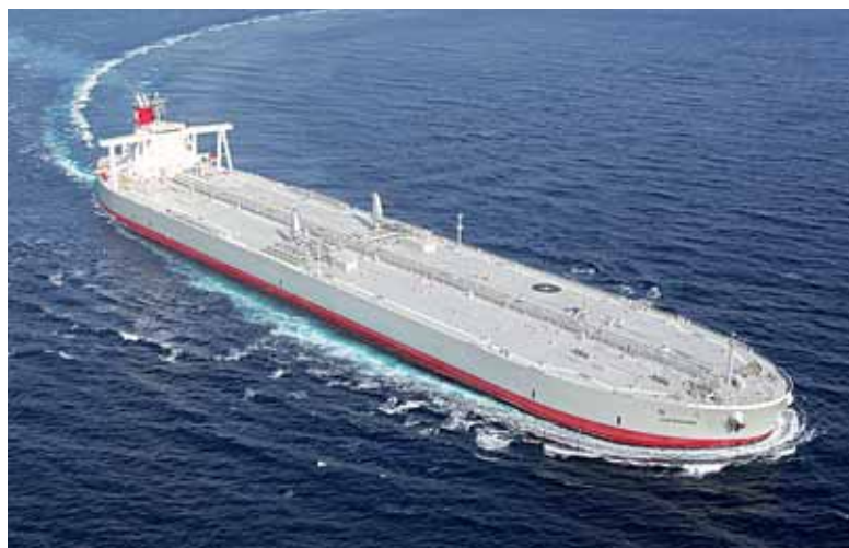
SAKURAGAWA Length/332.93m Breadth/60.00m Depth/29.00m Draft/20.305m DWT/299,982t Delivery/2009
