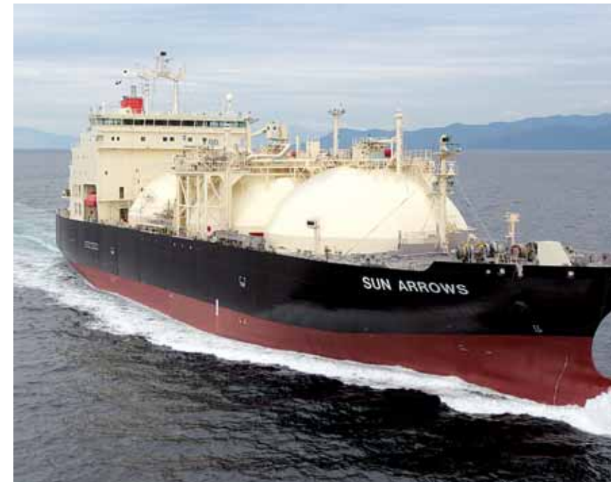
SUN ARROWS Length/151.00m Breadth/28.00m Depth/16.00m Draft/7.30m Tank capacity/19,468m 3 DWT/10,130t Delivery/2007
