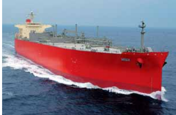
HISUI Length/226.00m Breadth/37.20m Depth/21.00m Draft/11.20m Tank capacity/80,199m 3 DWT/53,012t Delivery/2010
