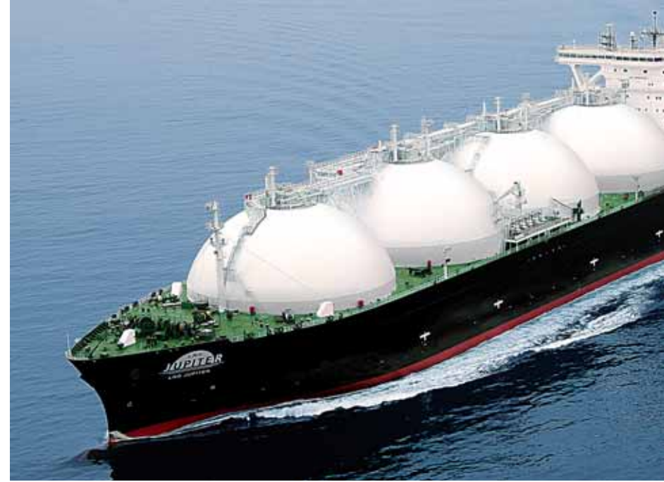
LNG JUPITER Length/289.50m Breadth/49.00m Depth/27.00m Draft/11.90m Tank capacity/155,999m 3 DWT/76,355t Delivery/2009
