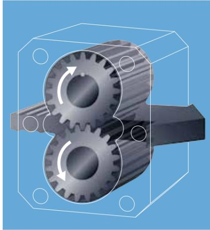
Liquid is filled in grooves of the revolving gears at the inlet, when the gears are disengaged.
