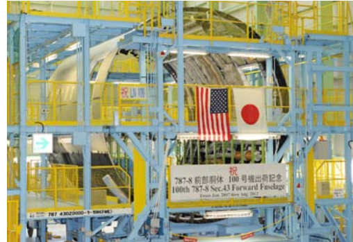
Forward fuselages for the Boeing 787
