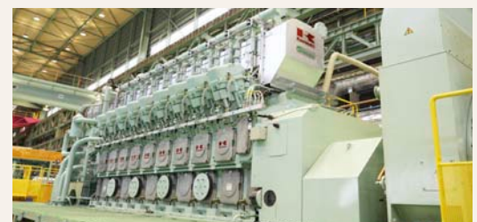
The Green Gas Engine boasts the world's highest power generating efficiency—49.5%.
