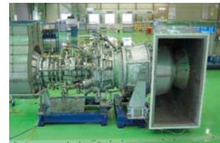
Gas Turbine “L30A”
