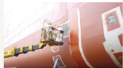
Welding inspection using an aerial work platform
