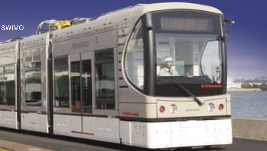
The LRV was named SWIMO (Smooth Win MOVER) because the goal was to realize (WIN) a vehicle (MOVER) with smooth (SMOOTH) boarding and exiting, and smooth entry into non-electrified segments.
