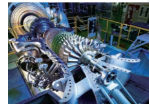
30MW-class gas turbine first shipped overseas
