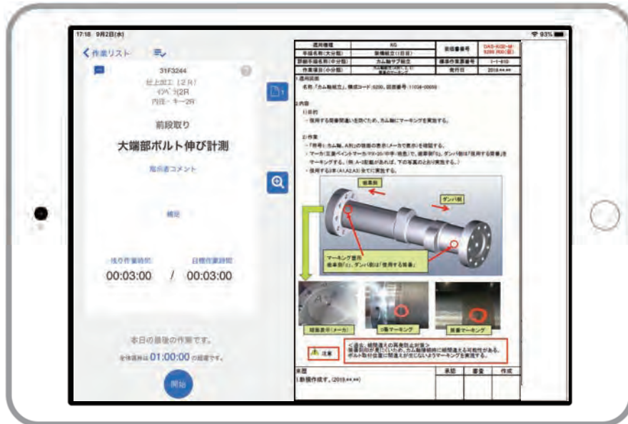
Fig. 3 Electronic production control board (OWL)
