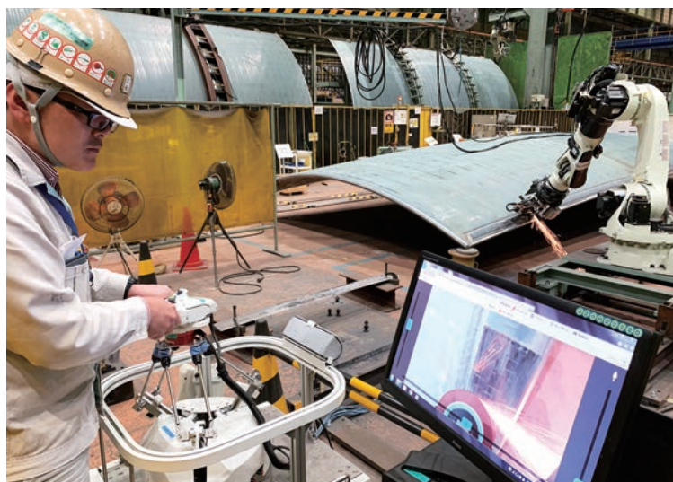
Fig. 5 Grinding operation using Successor-G
