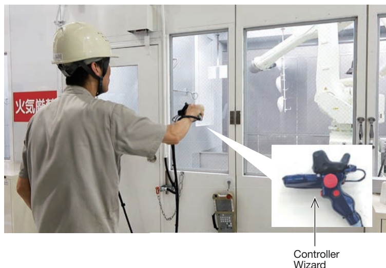
Fig. 4 Painting operation using Successor adapted for coating
