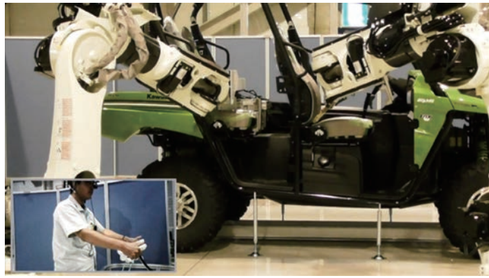
Fig. 1 Multiple robots remotely controlled by one worker
