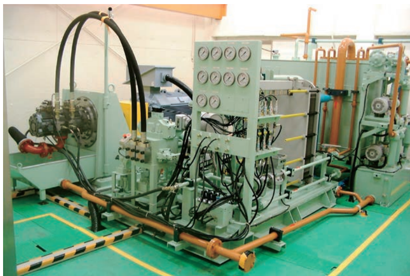
Fig. 1 Evaluation bench for hydraulic components HYPAM
