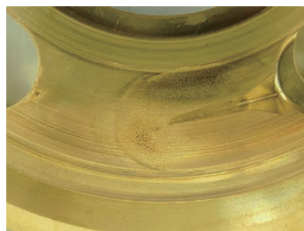
Fig. 2 Example of cavitation erosion on valve plate
