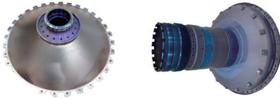
Fig. 1 Large forged parts produced with 50,000-ton press
