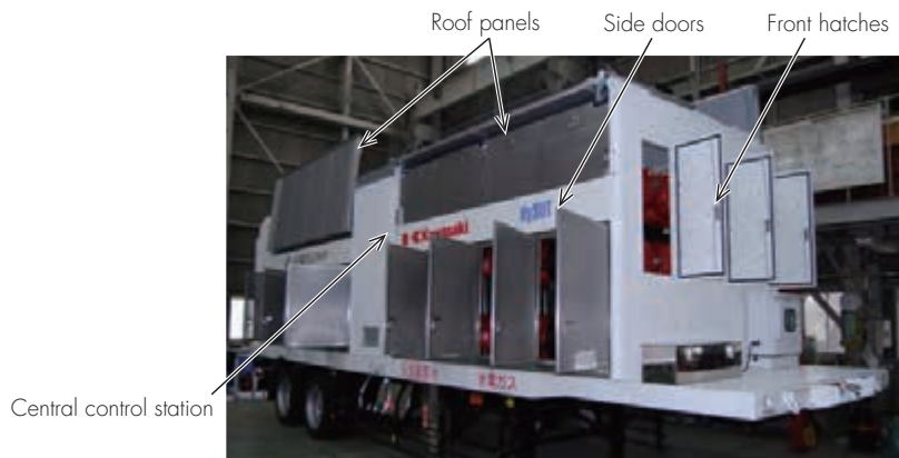
Fig. 3 Roof panels, side doors
