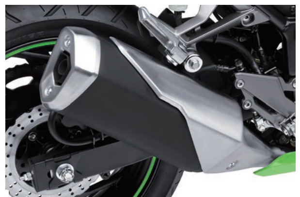
Fig. 7 Short muffler with complex cross-section
