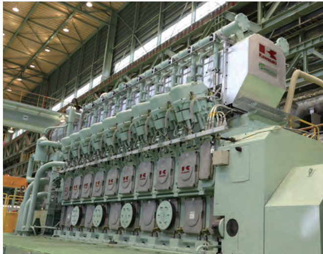
Fig. 7 7.8 MW Kawasaki green gas engine
