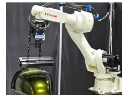
Visual inspection of complex curved surfaces
