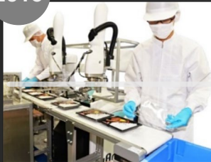
“duAro” dual-arm SCARA robot able to collaborate with humans
