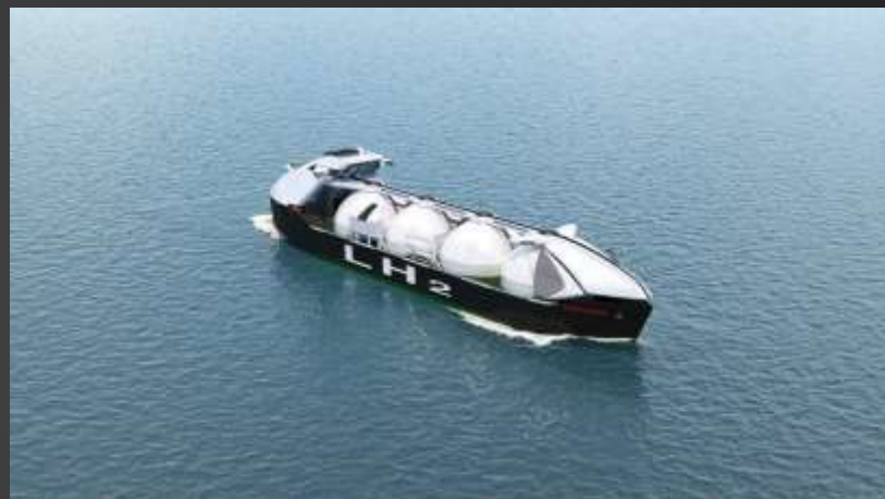
Liquefied Hydrogen Carrier (40,000 m 3 x 4 hydrogen tanks)
