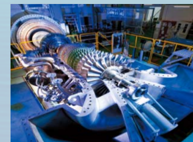
Hydrogen gas turbine
