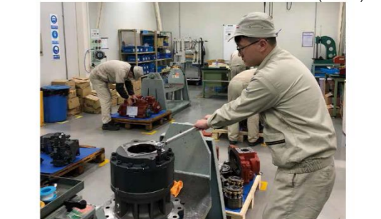
Overhauling hydraulic equipment at Kawasaki Precision Machinery Trading (Shanghai) Co., Ltd. CS
