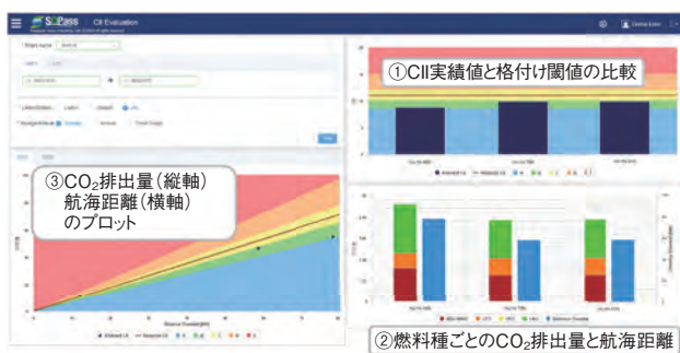
図5 CII評価情報の航海ごとの表示 Fig.5 Representation of CII evaluation information for each voyage
