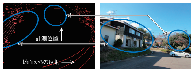
図5 レーダ取得データと写真の対比 Fig. 5 Comparison between data acquired by radar and photo
