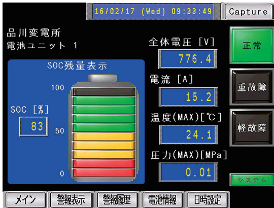
図2 蓄電池監視画面 Fig.2 BPS monitoring screen
