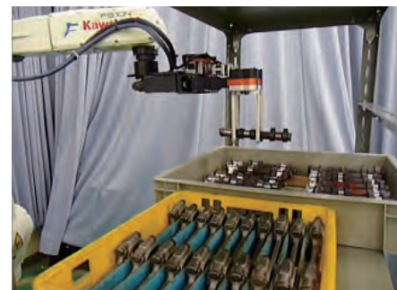
図8 棚への侵入 Fig.8 Entry into space between shelves
