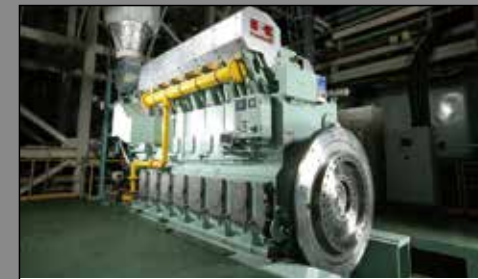
Marine gas engine (Kawasaki Green Gas Engine)
