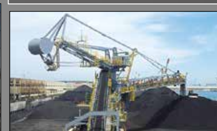
Stacker-reclaimer for transporting coal
