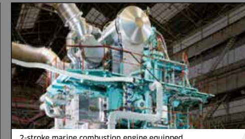
2-stroke marine combustion engine equipped with combined low emission system K-ECOS
