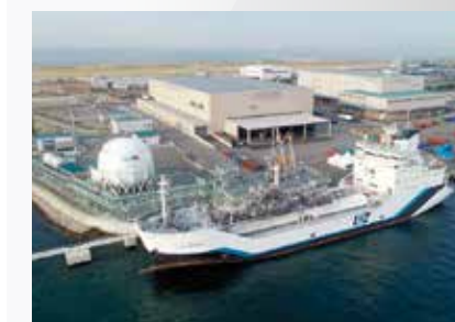
The world's first liquefied hydrogen carrier SUISEI FRONTIER and handling terminal "Hy touch Kobe"
