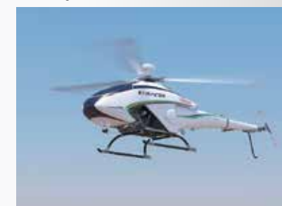
Vertical take-off and landing aircraft (VTOL) K-RACER™ (Kawasaki Remote, Autonomous and Cargo-ability Enhanced Rotorcraft)
